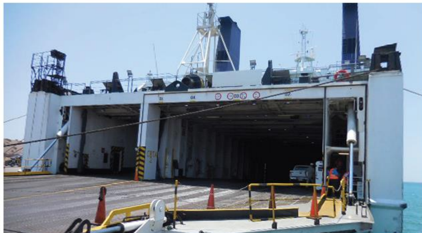
Figure 4: MV Cabo Star showing Stern Ramp Loading Deck
