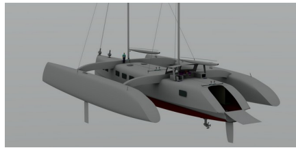
The Alpha Zulu RoPAC Class — sub-500 GT sail-electric passenger-cargo trimaran, wind-primary with retractable electric propulsion.
