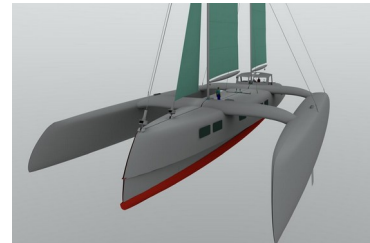
The Alpha Zulu RoPAC Class — sub-500 GT sail-electric passenger-cargo trimaran, wind-primary with retractable electric propulsion.
