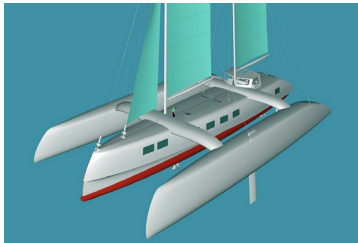
The Alpha Zulu RoPAC Class — sub-500 GT sail-electric passenger-cargo trimaran, wind-primary with retractable electric propulsion.
